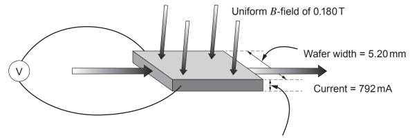
Wafer thickness = 0.400 mm
